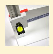
The Abdominal Caliper has a built-in level. If you desire to use the level, the bubble must be perpendicular to the measurement arm. The bulb can be removed by carefully sliding upward. Turn the bulb and slide it back onto the measurement bulb as shown at left.
