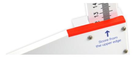
**Note:** The Caliper must be read from the top of the measurement arm where the red line is drawn.
